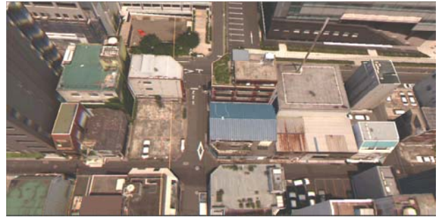
Figure 9. Referenced 3-D data (precise 3-D data) constructed from three-line sensor images
