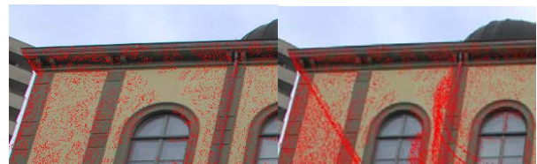
Figure 3: Close-up of a back projection without HPR Figure 4: Close-up of a back projection with HPR
