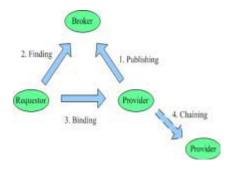
Figure 1 Service Oriented Architecture
