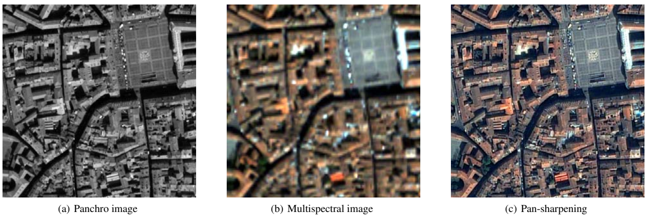
Figure 4: Pan-sharpening example: high resolution of the panchromatic image is introduced in the multispectral image to obtain a multispectral high resolution image with a basic method.
