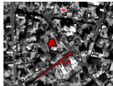
Figure 2: Segmentation example: from three different seeds. The fast marching algorithms generates three different areas.
