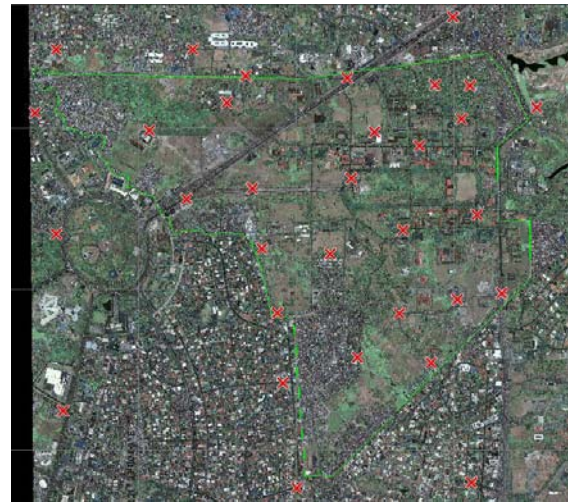
Figure 2. UP Campus Base Map Showing Boundary and Distribution of GCPs in the Project Area
