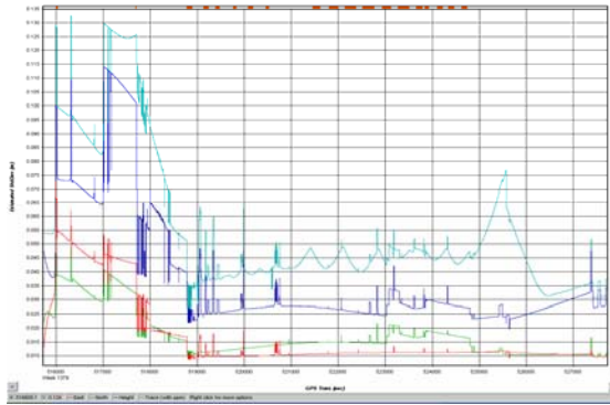
Figure 13. Using GPS to resolve the orbital position in three-dimensional space precision analysis ( xy < 2\text{cm} , z < 4\text{cm} )
