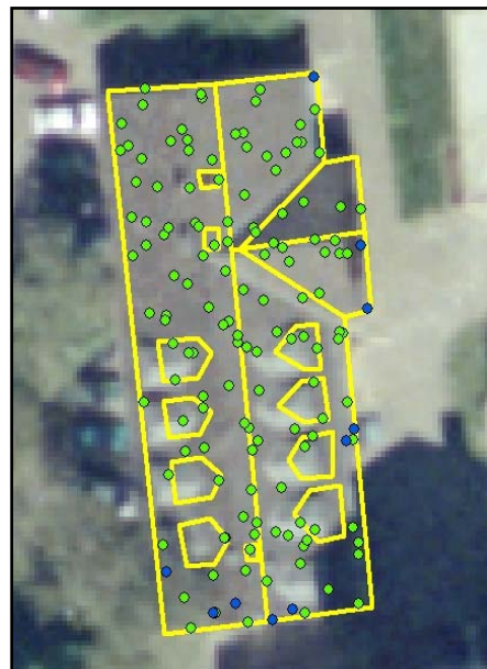
Figure 6. DSM measure points that represent the ground surface height inside the roof's outline are eliminated by a 3m threshold value (blue points)
