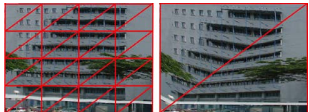
Figure 5. Geometrically corrected facade texture from Figure 4. High resolution mesh (left). Low resolution mesh (right).
