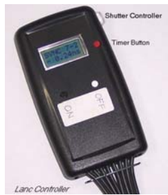
Figure 6. External shutter device to control the stereo cameras
