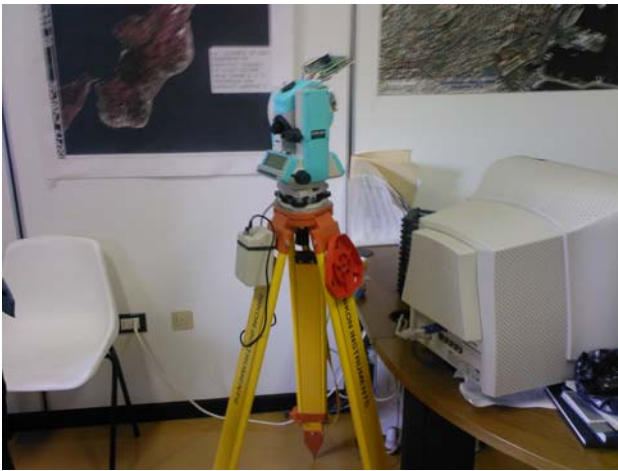
Figure 6. The instrument used for positioning the MEMS INS
