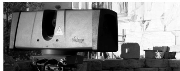
Figure 5. The Surphaser ® 25HSX laser scanner
