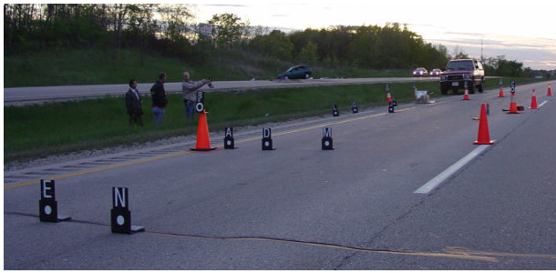
Figure 3. 'Evidence markers' placed on features of interest, note the large letters for easy identification.
