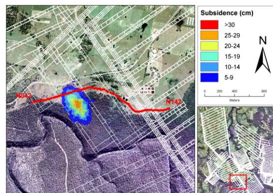
Figure 9. DInSAR height change derived from ascending ALOS images acquired on 27 Dec 2006 and 11 Feb 2007 (46 days apart) and overlaid on Appin Mine plan.
