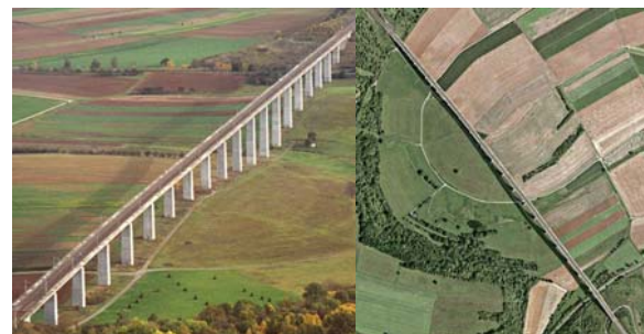
Figure 4: Images of a railroad bridge made of concrete-steel near the city of Zellingen in southern Germany, (left) oblique photo taken out of the aircraft with a consumer grade camera, (right) optical image from GoogleEarth.
