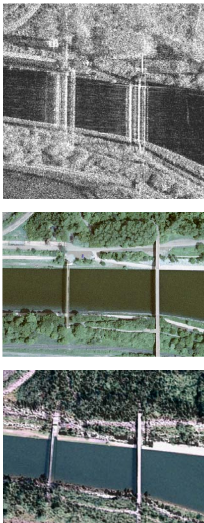
Figure 1: Test images of bridges near the city of Dorsten in southern Germany, (top) InSAR magnitude image pair taken in X-Band (illumination direction from right to left), (centre) optical aerial image, (bottom) 3D visualization of optical and InSAR data after fusion.
