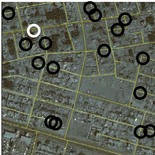
Figure 7. Road blocks, Black circles: correct detection, White circle: wrong detection
