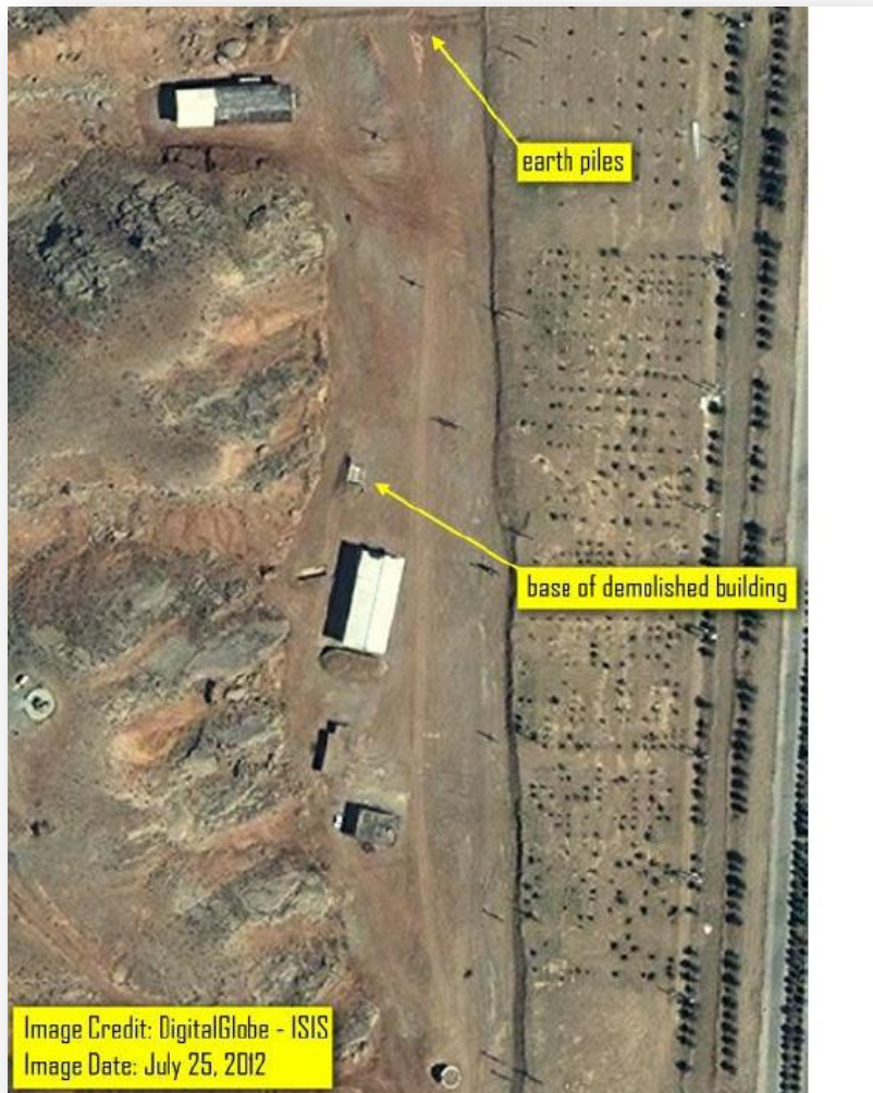
Figure 2. Satellite image from July 25, 2012 showing the results of extensive alterations undertaken at the suspected high explosives testing site, including the demolition of two buildings and major earth displacement activities.
