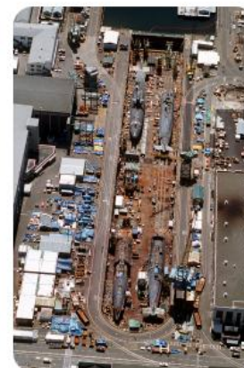
Aerial view of four decommissioned nuclear-powered attack submarines in the late stages of being scrapped out in a graving dock
