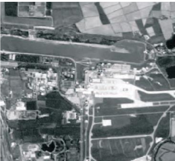
Figure 6: Optical image of Linate Airport taken from the SPOT satellite. No speckle is visible and the fields that surround the airport look homogeneous
