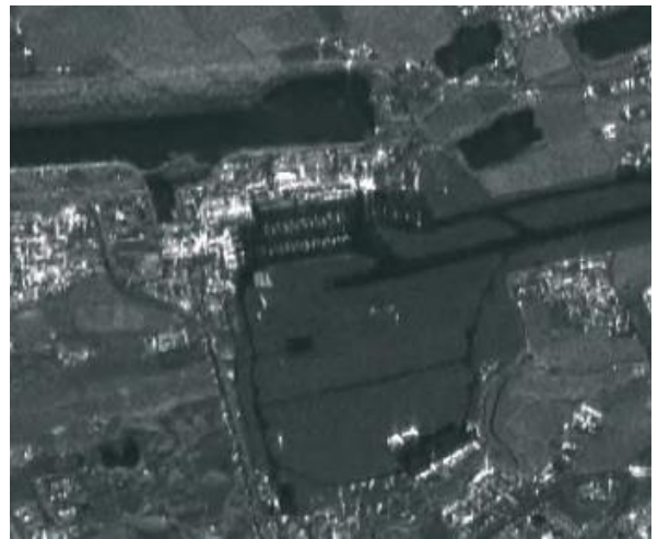
Figure 7: Average of multiple ERS SAR images of Linate airport: the speckle effect on the homogeneous fields around the airport has disappeared.
