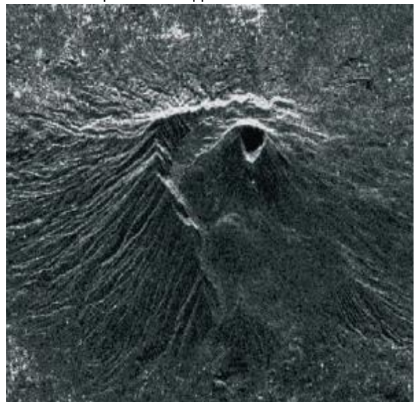
Figure 8: ERS-2 SAR image of Mount Vesuvius (Italy), as detected. The slant range direction is vertical on the image (near range is in the upper part of the image). Brighter levels correspond to stronger backscattered radiation.
