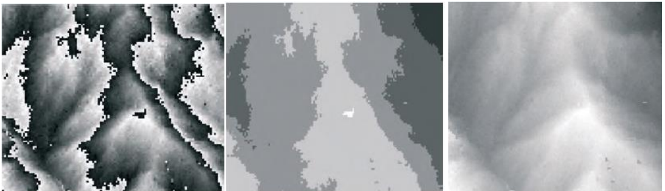
Figure 4: Left: SAR interferometric phase generated by means of two ERS images. The 2\pi phase discontinuities are clearly visible as black/white transitions. Middle: Unwrapped phase. Right: The 2\pi phase discontinuities have been eliminated by adding or subtracting an integer multiple of 2\pi to each pixel of the original interferometric phase image.
