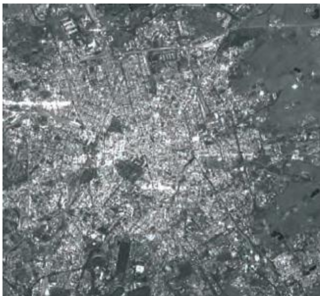
Figure 2: ERS SAR detected image of Milan (Italy). The image size is about 25 km in ground range (vertical) and 25 km in azimuth (horizontal).
