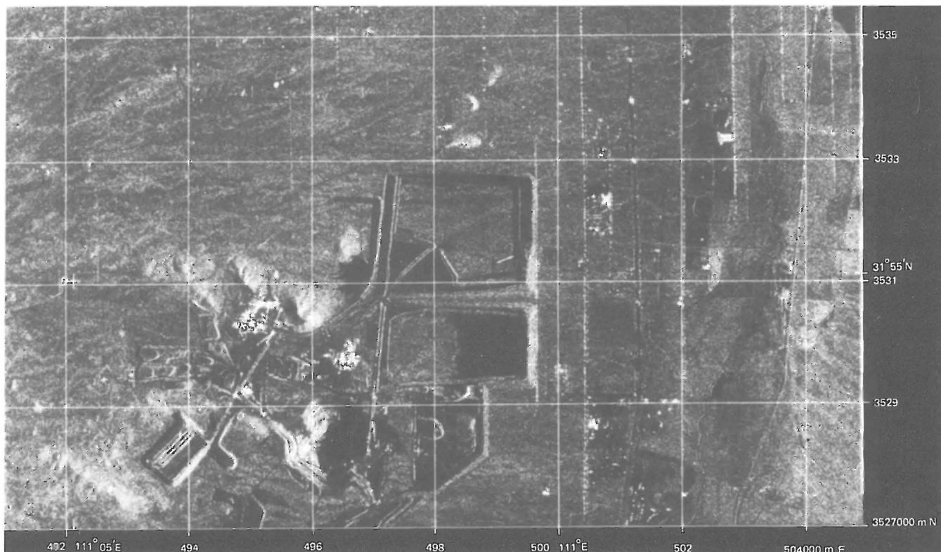
Figure 1: Example of a radar orthophoto of Sierrita, Arizona, USA (Section). Produced on Wild Avioplan OR-1 from X-band Goodyear GEMS images (Leberl et al., 1980).
