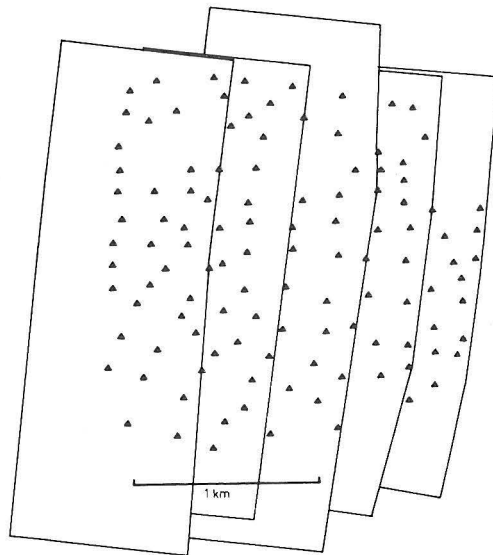
Fig. 1. The control net of Jämijärvi test field and the aerial photography.
