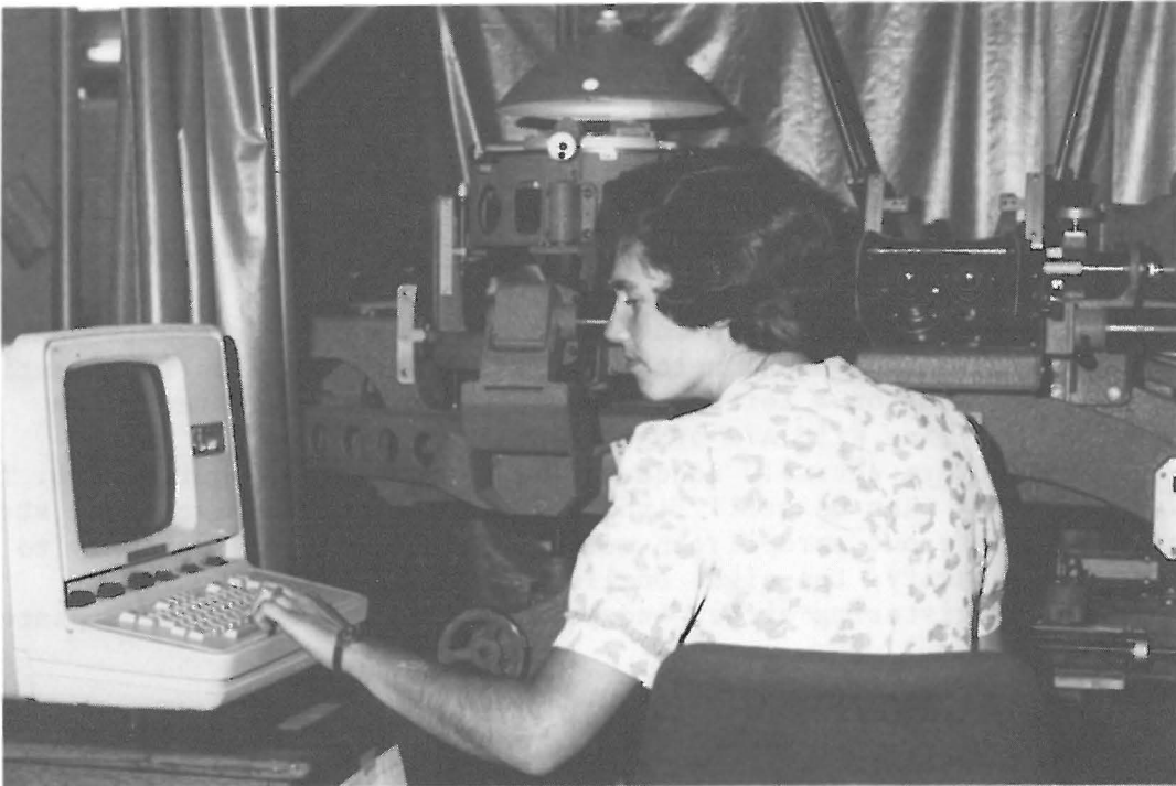
FIGURE 2. On-line stereoplottor and visual display unit
