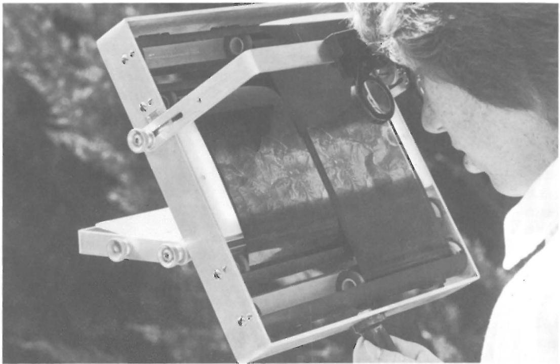
Figure 3. Using a microfiche viewer to stratify bark beetle infestation on optical bar film.
