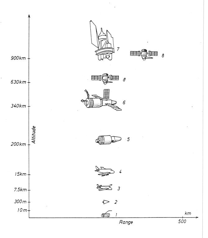
Fig.1. 1- spectrometric measurements, 2- hang glider, 3- air-craft AN- 30, 4- aircraft, 5- KOSMOS, 6- SALUT -7, 7- LANDSAT, 8- METEOR -Priroda.
