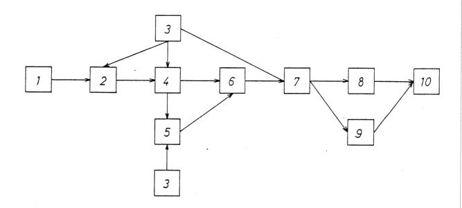
Fig.2. 1- data acquisition, 2- photolaboratory, 3- power supply 4- microdensitometr, 5- colour composite, 6- data interpretation, 7- field checking, 8- spectrometric measurements, 9- ground sample acquisition, 10- photointerpretation and key elaboration.
