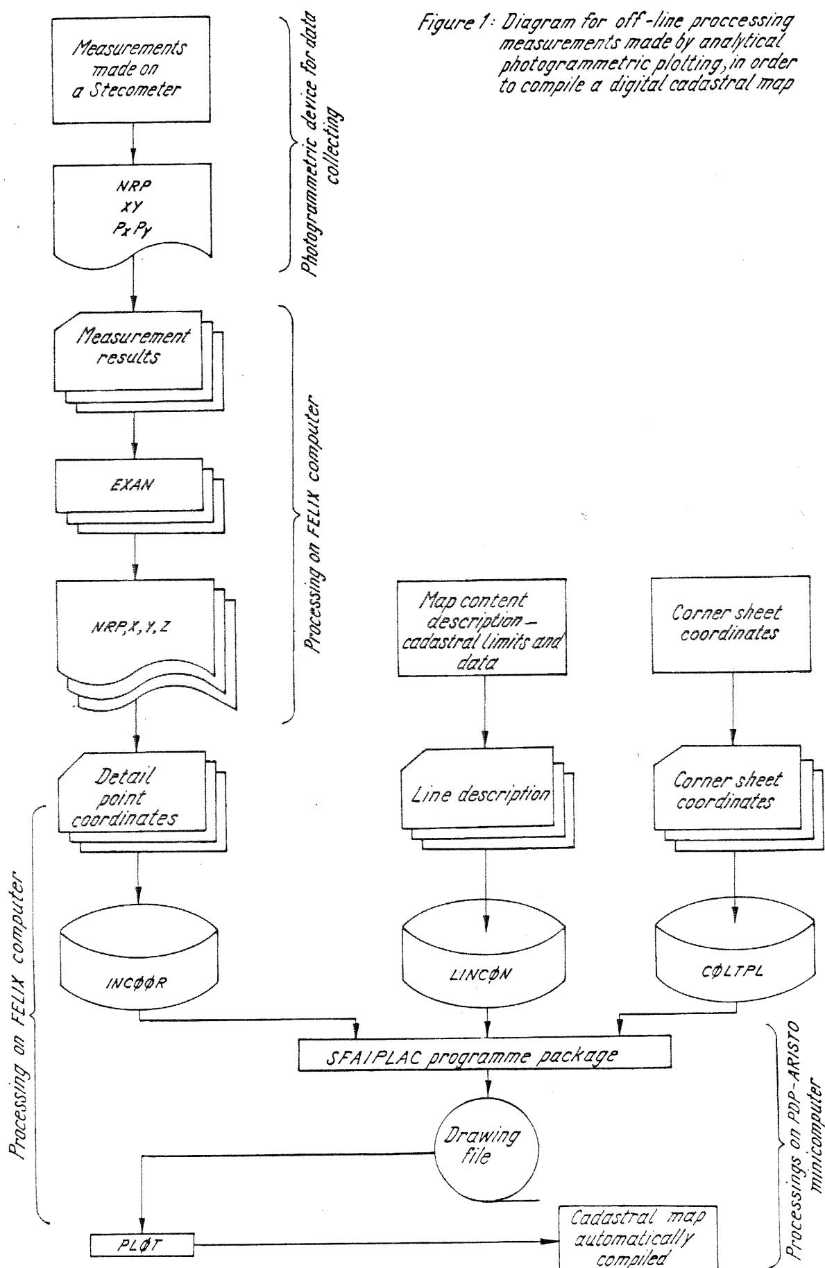
The automatic photogrammetric system for cadastral mapping (SFAIPLAC), which is the object of this paper, was designed to use input data obtained by analytical photogrammetric plotting (measurements made on a Stacomter and recorded on a G - type Coordinate) to process data in a FELIX - C - 256 computer and to display results as a graphical representation, using ARISTO plotter (Figure 1).
