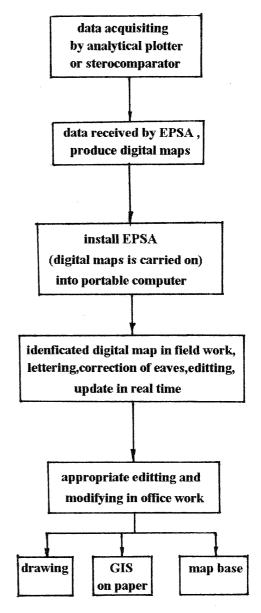
The main points of the new method are: the digital map can be produced from aerial films directly; EPSA identificating and mapping in the field work; editting, updating and lettering in real time. It ensure the perfectness and correctness of maps. After approciate editting and modifying in office work, the maps can be plotted on paper, or transferred to GIS, or input to mapbase.
