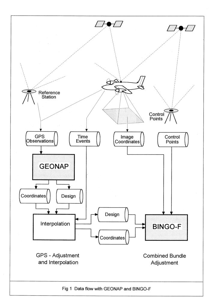
introduced into the BINGO-F adjustment. This unknown stands in the BINGO-F adjustment until a new (resolved or unresolved) ambiguity occurs for this satellite.
