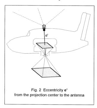
The last step after the computation of the aircraft's GPS antenna position is the interpolation of the camera exposure events between the GPS exposure events. The reduction from the GPS antenna position to the camera's projection center is also done in this step. BINGO-F enables the estimation of the vector  $\mathbf{e}$ ' from the projection center to the antenna (see Fig. 2) as additional unknown in the adjustment process.
