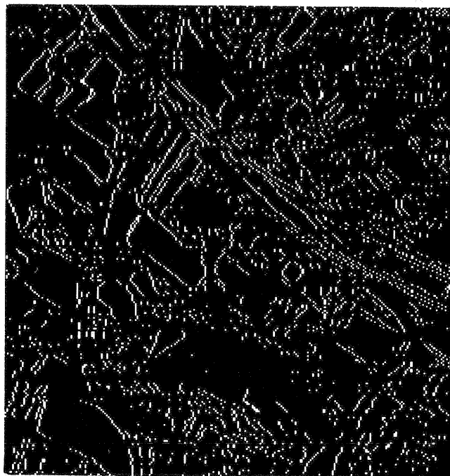
Fig. 6: The useful linear features extracted by string matching (left image)
