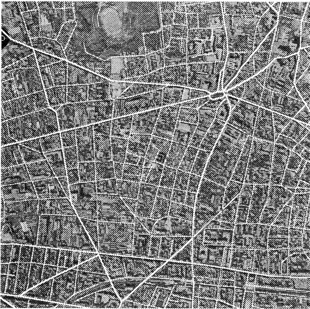
Fig. 3 - The road network extracted from the map is superimposed on the aerial left image.
