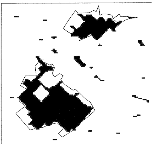
Figure 3: Segmentation of image objects (settlement) by morphology operators (black contour line: original DLM200 objects)
