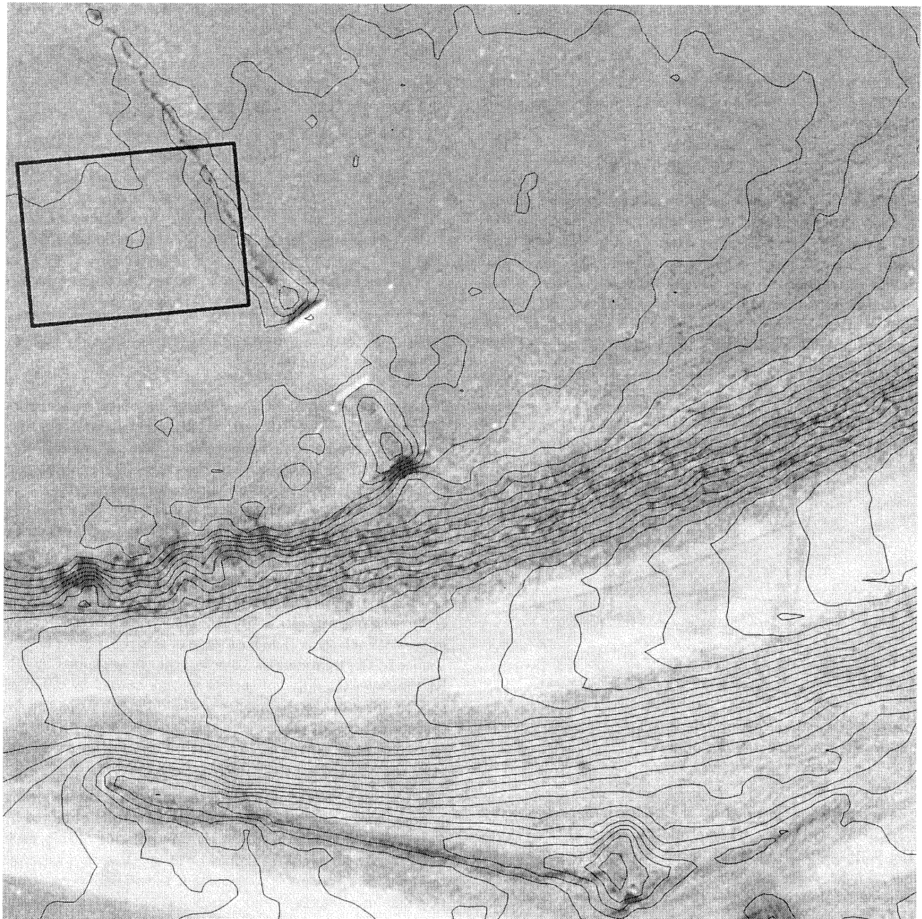
▲ Fig. 2a: Orthoimage and contours, surface reconstruction using 3 images orthoimage scale: 1 : 300 equidistance of contours: 0.2m
