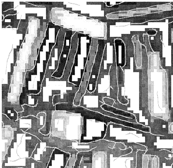
Figure 5: Boundary pixels rendered with mean pixel value of region (white pixels are interior pixels), edgel chains superimposed
