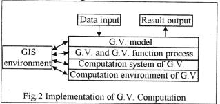
model, the processing about graphical variables is divided into four logical layers. Each layer performs a related subset of the functions required to support the
