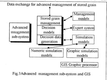
currently used in 2D-SGMS for managing and processing the spatial data and graphical variables. Advanced management subsystem of 2D-SGMS is shown in Fig. 3, which is based on an application model
