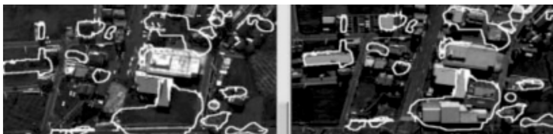
Figure 7. Detecting house changed areas by Gradient Direction Histogram Analysis
