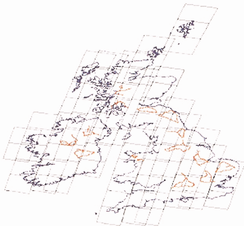
Figure 2 ERS Tandem IfSAR pair strips and frame boundary footprints (black) for the first-pass DEM generation, with kGPS tracks superimposed (red). There is only one IfSAR pair per footprint in the first-pass coverage
