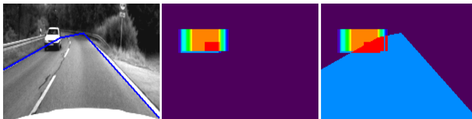
Figure 5: Oncoming traffic (image with lane-information, movement-sensitive representation without and with preactivation). The preactivated region is determined by the lane information. The value indicates the grade of activation.
