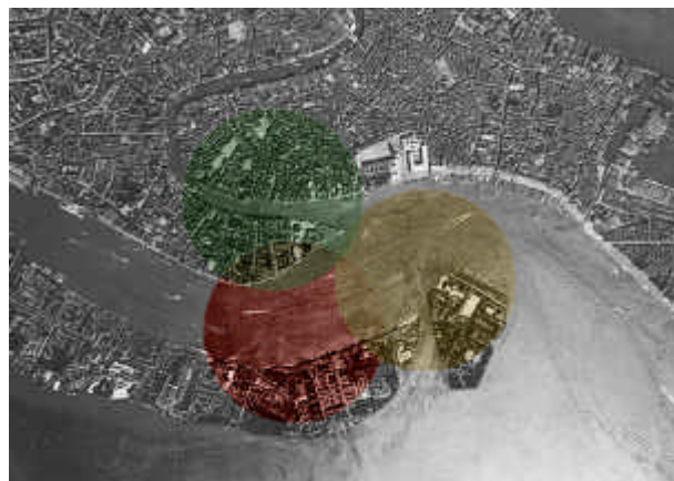
Figure 5-6. Simulation of a aerial photography from aeostat from 750m with a 150mm camera. At left, the image on the plate with the total field and the usable field marked; at right a recovery hypothesis.
