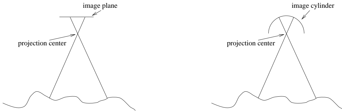
Figure 1: Two projections. On the left the focusing surface is a plane and on the right a cylinder.
