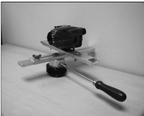
Figure 2: Camera mounted on a special rotation tool.
