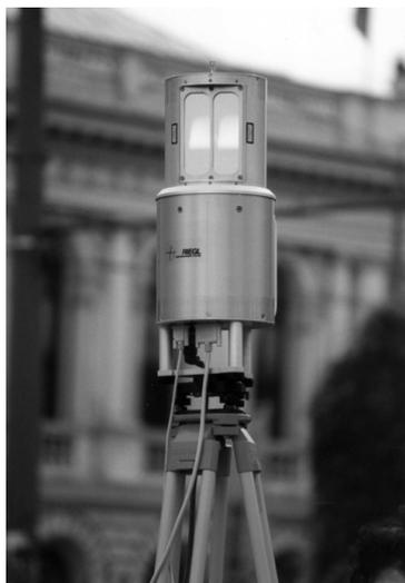
Figure 1 – The LMS-Z210 laser-scanner
