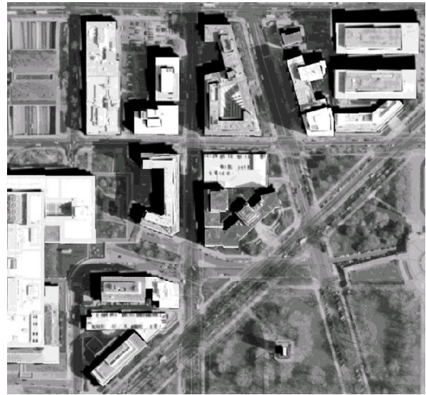
Figure 14: True orthographic mosaics can be generated on the fly in real time by simply taking an orthographic overhead view of a scene that uses virtual projectors. This ortho view of the scene from Figure 2 also highlights the occlusions caused by the buildings.
