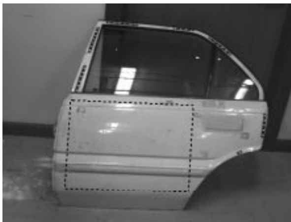
Figure 4: First test object, a car door, with the measured surface area indicated by the dashed line.
