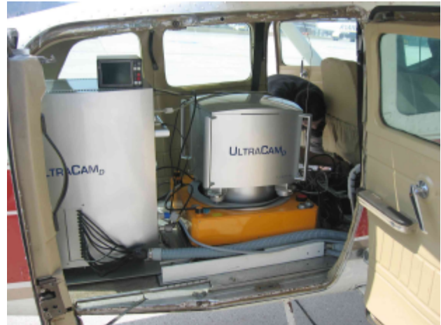
Fig. 4: Installation of the ULTRACAM D in the Cessna 206 survey aircraft
