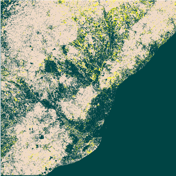
Figure 2: 2003 SPOT Image following supervised maximum likelihood classification (occupied area; green area; and soil) © SPOT Image Copyright 2003, CNES
