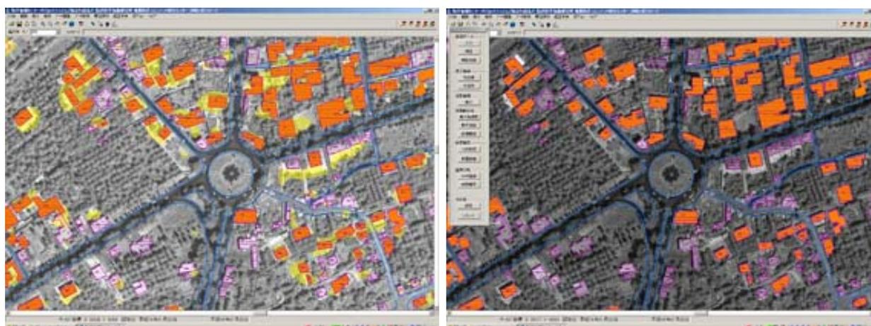
Fig. 12 Damaged house detected by comparison of Quickbird image data before and after
