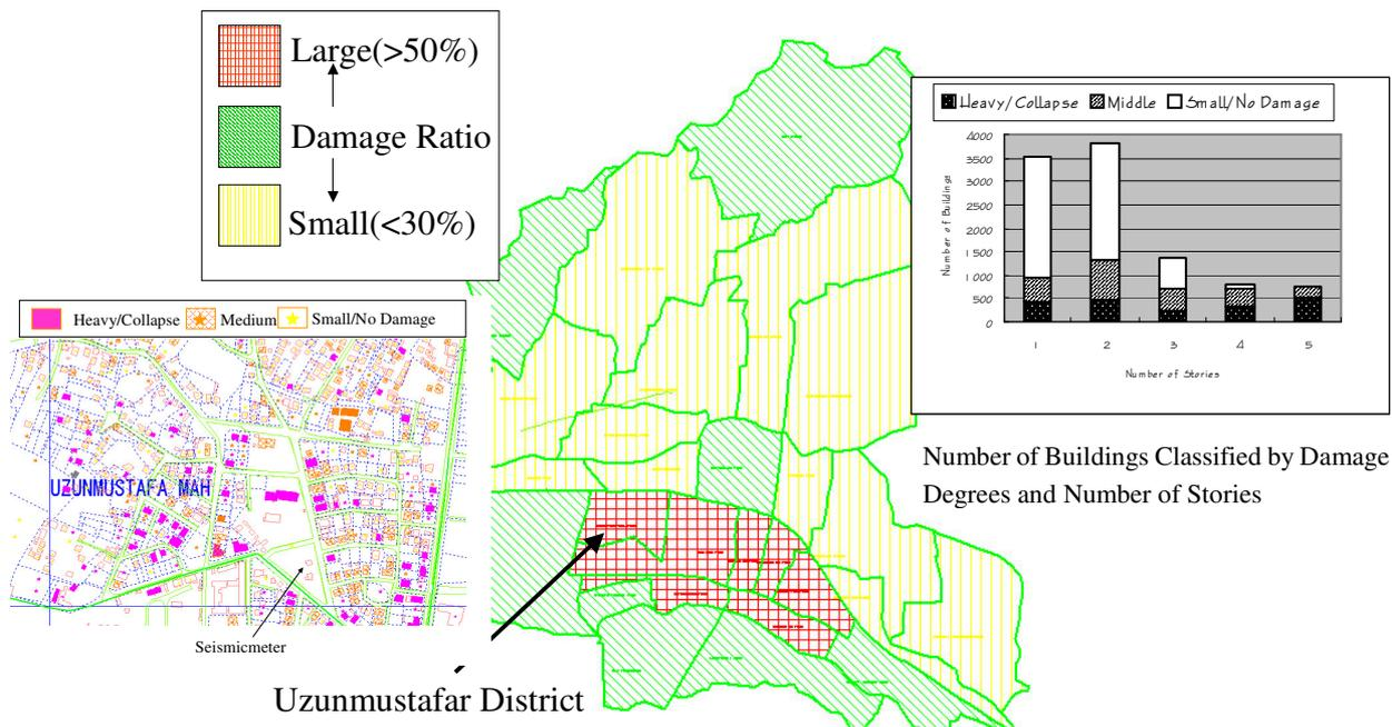
Fig. 9 Building Damage Status after the Second Earthquake
