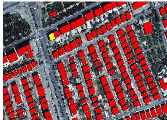
Figure6. Production of Buildings as Vector Layer
