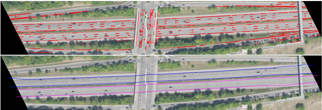
Figure 3. Example for road extraction at A96 exit Munich-Blumenau (clipping from nadir image). Upper panel shows line detections at a flight height of 1000 m, panel below shows the resulting road area after smoothing / gap filling.
