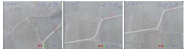
Figure 6. An object tracking result of airborne video using Mean-shift method
