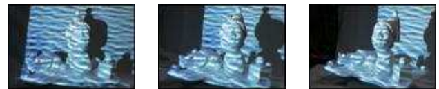
Figure 12: Examples of the image sequence acquired with a linear camera motion (253 textured images)
