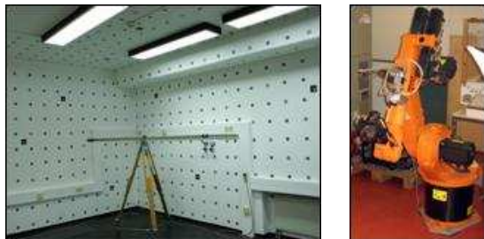
Figure 2: Control point field for camera calibration and the KUKA robot arm with the mounted digital camera.
