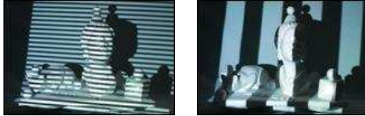
Figure 14: Examples of binary coded textures (9 images with horizontal and 10 images with vertical stripes)
