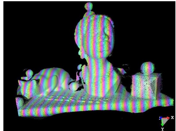
Figure 18: Reconstruction result of an implementation of the narrow-baseline stereo algorithm
