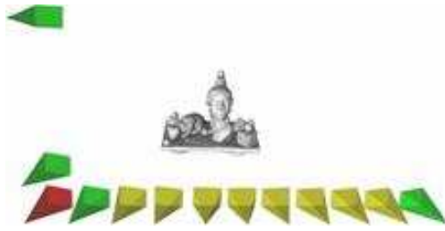
Figure 5: Orientation of the reference image (red), narrow- and wide-baseline stereo images (green) and the linear motion sequence (yellow).
