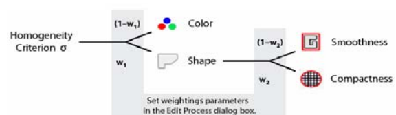
Figure 2. Weighted components of the homogeneity criterion (Definiens, 2007)
