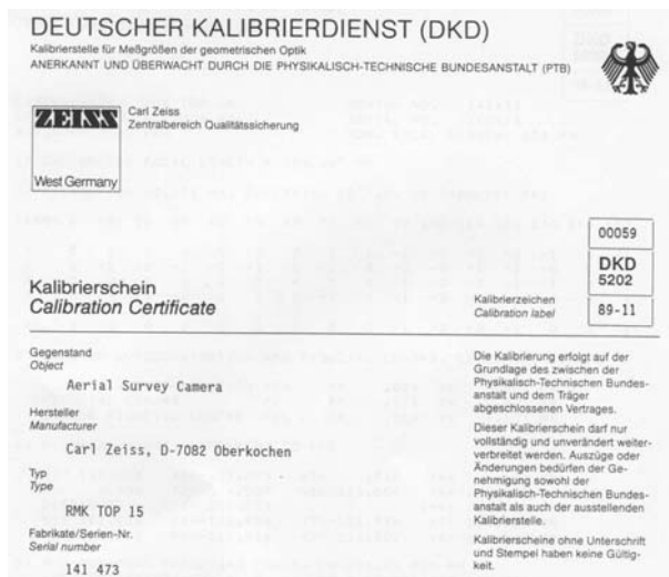
Fig. 7.49: Certificate (head) for the camera calibration at CARL ZEISS, Oberkochen, authorized by the PTB
