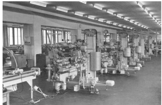
Fig. 4.16: Serial production of the STEREOPLANIGRAPH in the MJ 6 photogrammetric assembly hall (1952)
