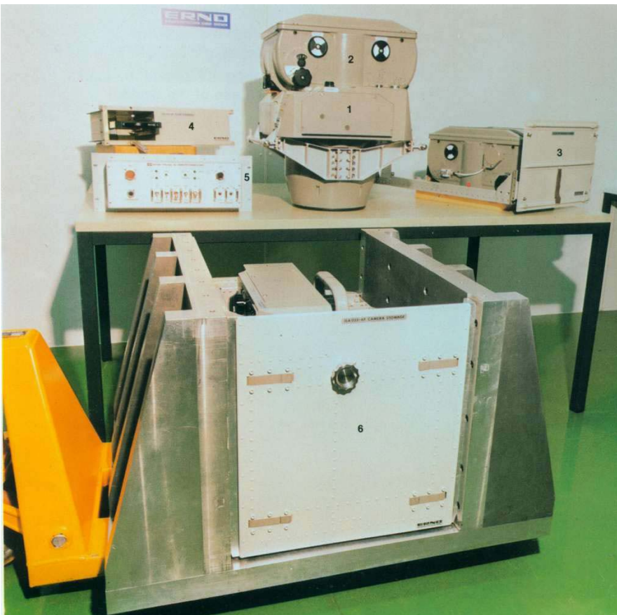
Fig. 7.22: METRIC CAMERA equipment with camera body (1), film magazine (2), additional magazine in drawer (3), camera filter in box (4), remote control (5) and camera container (6)
