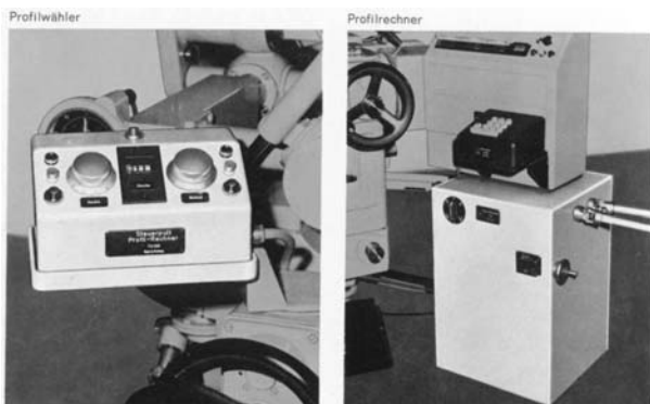
Fig. 10.39: Profile setting at the C 8 and profiling gearbox between C 8 and the motor drive at the Z 2
