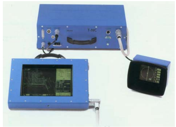
Fig. 7.38: T-NC navigation computer with touch-screen-display for the navigator and with pilot's display
