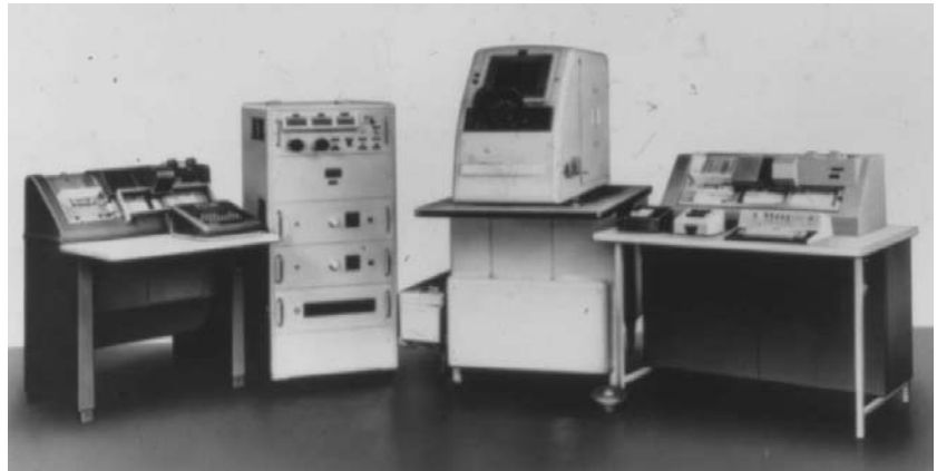
Fig. 9.32: PEK precision monocomparator with card punch and pre-positioning from card reader
