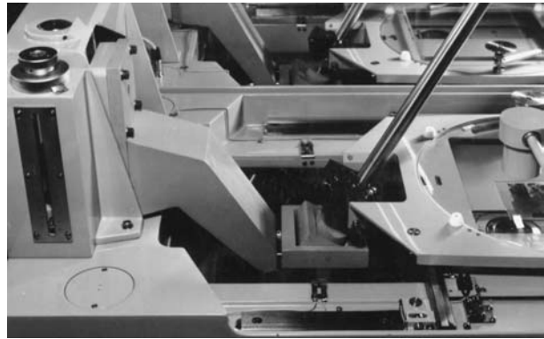
Fig. 10.22: Optional projection cardans for the use of (terrestrial) focal lengths <84 mm
