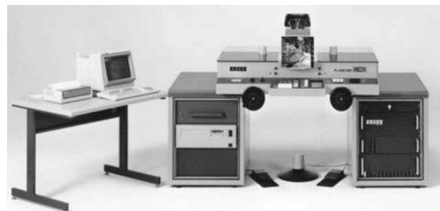
Fig. 11.29: C 140 PLANICOMP with HP 1000 A 600 computer, without cabinet doors (1985)
