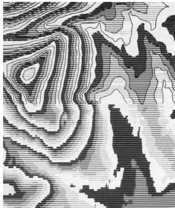
Fig. 8.17: HS dropped line output of the GZ 1, partly with manual derived contour lines
