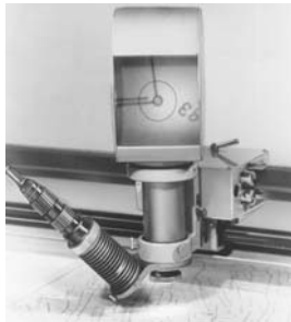
Fig. 10.38: Viewing device for the Z 2 coordinatograph with 10x magnification
