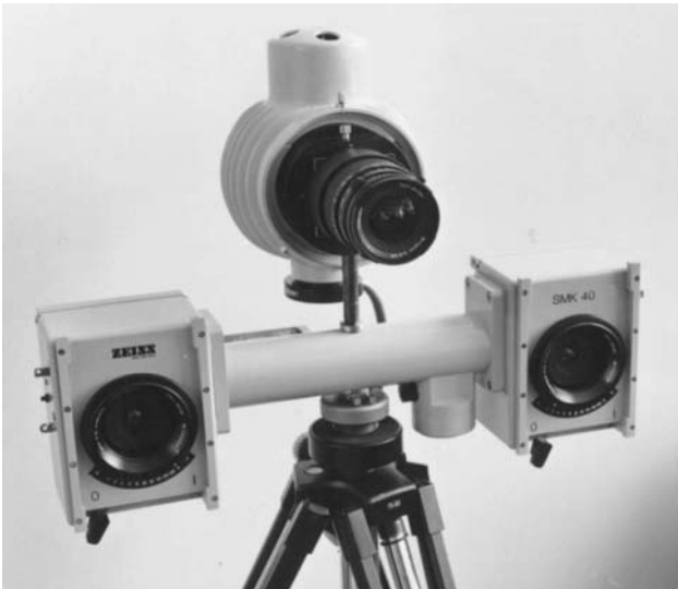
Fig. 13.3: SMK 40 with texture projector (1984)
