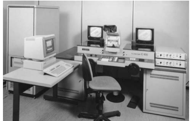
Fig. 11.30: C 100 PLANICOMP with digital image correlation
