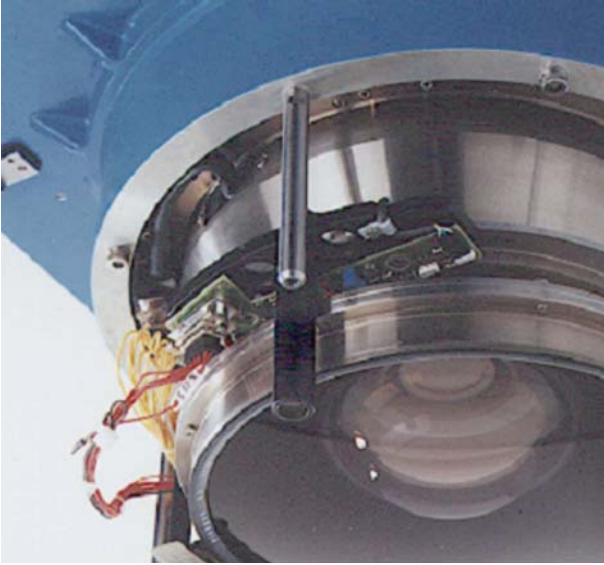
Fig. 7.31: Sensor head of the NA automatic navigation near RMK TOP lens
