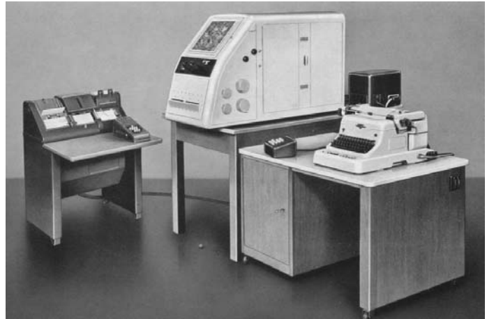
Fig. 9.24: PSK precision stereocomparator with ECOMAT II (1960)
