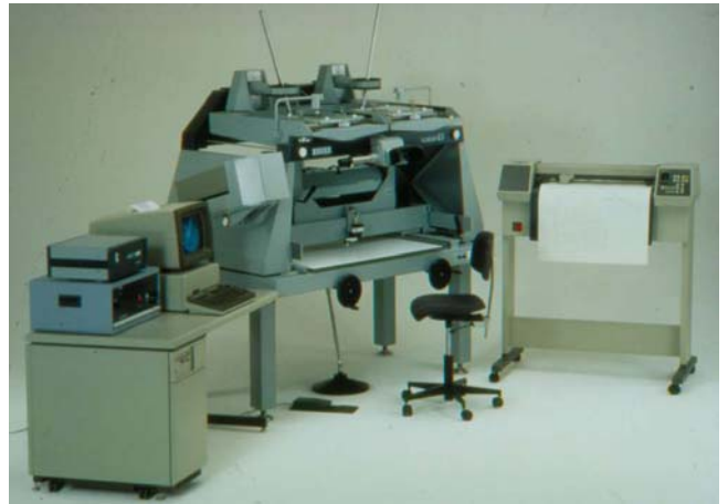
Fig. 10.58: E 3 PLANICART for software-supported mapping with graphical superimposition and HP 7580-Plotter (1984)
