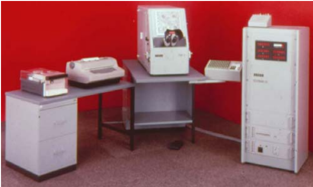
Fig. 9.34: PSK 2 with point numbering unit 2, automatic typewriter and paper tape punch (1971)
