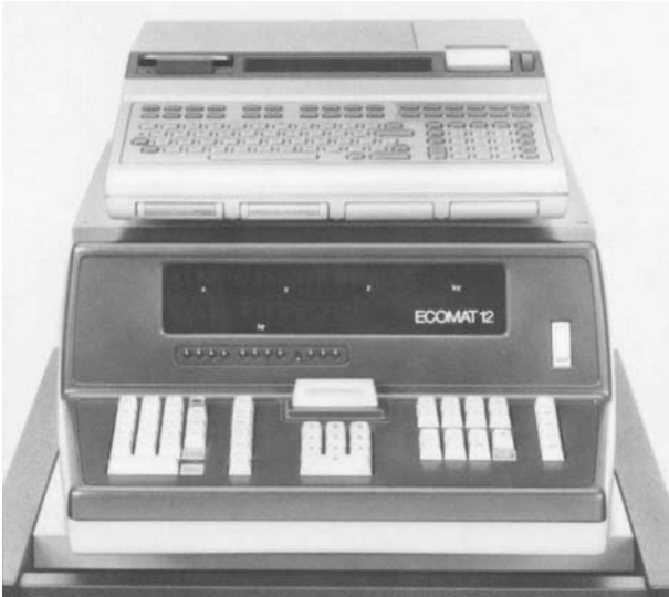
Fig. 9.16: ECOMAT 12 with additional programm buttons and HP 9825 desk computer
