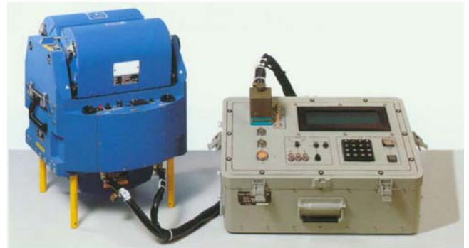
Fig. 15.12: KS-153A with LM-230A automatic test unit
