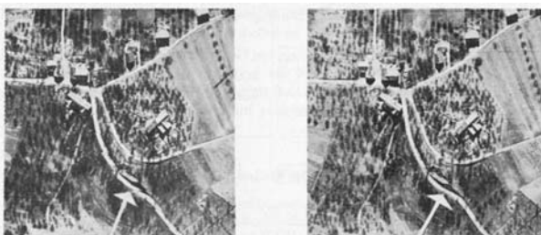
Fig. 8.15: Image improvement by optical interpolation (clippings with and without mismatches)
