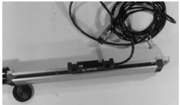
Fig. 9.10: Incremental linear encoder for the ECOMAT 11
