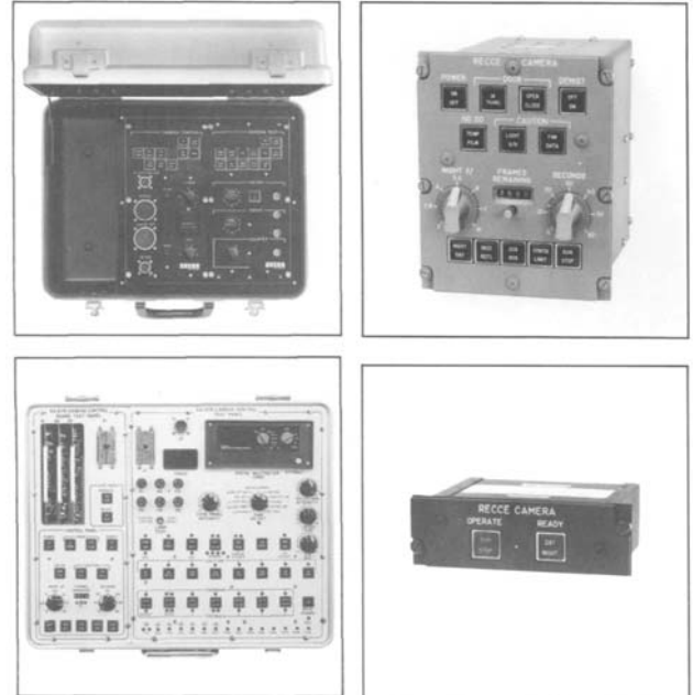
Fig. 15.6: Test sets and control panels for the KRB 8/24
