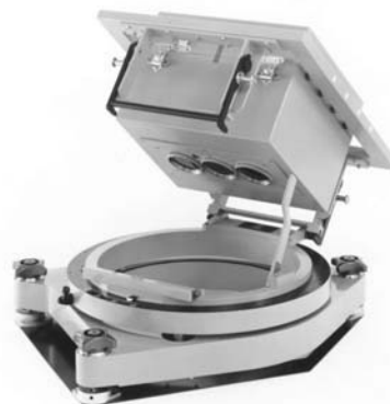
Fig. 15.17: MUK 8/24 multispectral camera from ZEISS with adapter and AS II mount of the RMK (1972)
