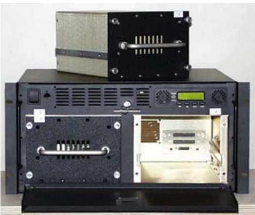
Fig. 7.48: DMC storage device (1st generation): MDR mass data recorder with 2 units with each 146 GB capacity
