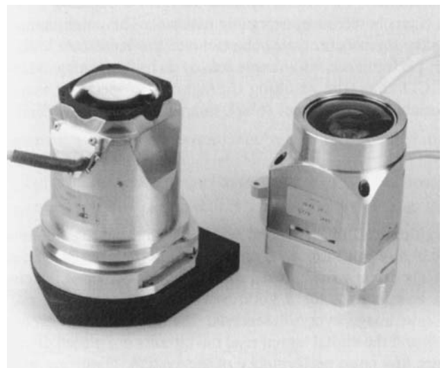
Fig. 7.41: Camera heads for the panchromatic (left) and for the colour channels (right)
