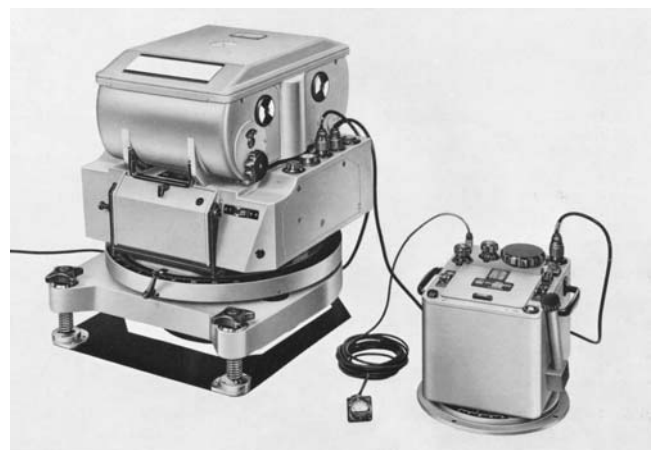
Fig. 7.2: RMK A 15/23 in AS II mount together with IRU and the pilot's display for time of exposure (1961)
