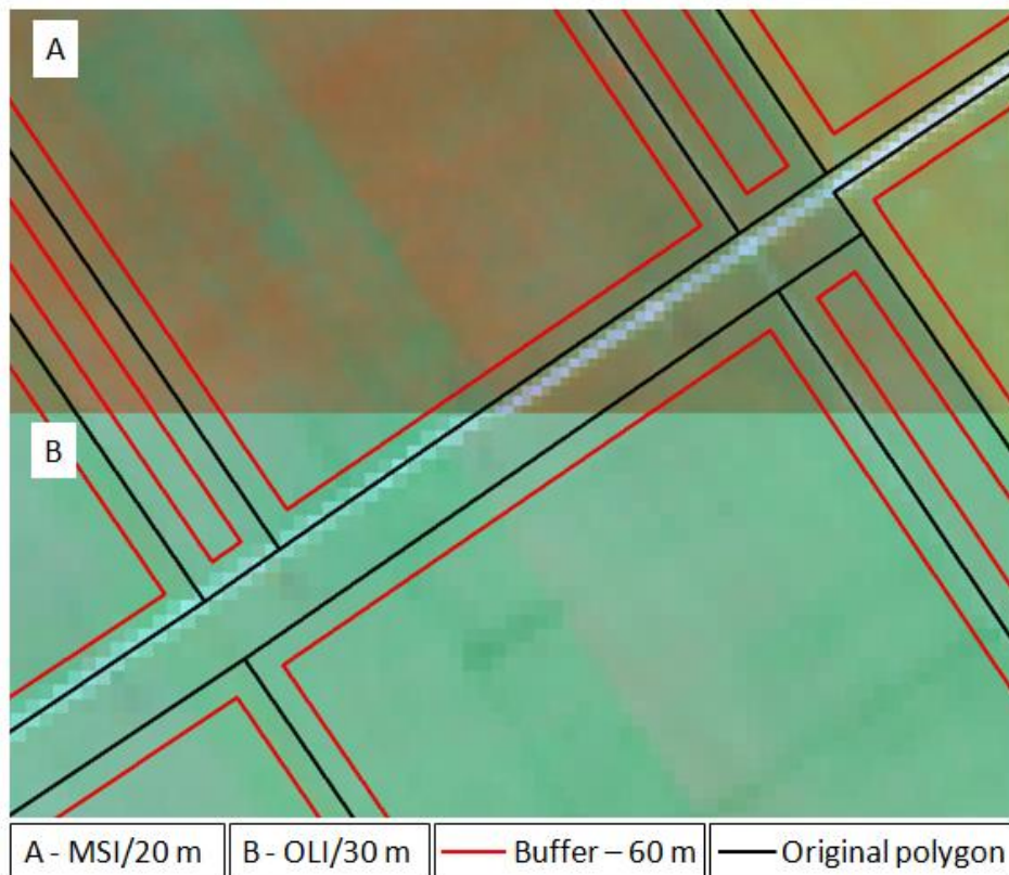
Figure 7. Illustration of crop field boundaries over false-colour compositions of (A) Landsat-8/OLI and (B) Sentinel-2/MSI images. In black are the original polygons and in red the final boundaries considering a buffer zone of 60m.
