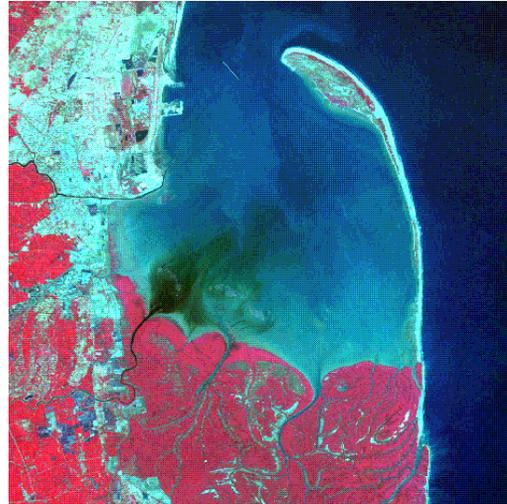
Fig. 7. A plume from a sugar factory and its dispersion (dark colour) in the Kakinada Bay, Eastern India.
